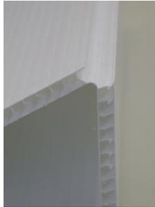
..... Note only the top layer of plastic is cut to allow the board to fold
